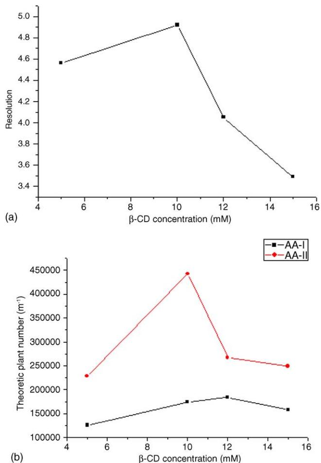
Fig. 3. Effect of  $\beta$ -CD concentration on resolution (a) and theoretic plate number (b) of AAs. Separation conditions: borate buffer (pH 9.2), 50  $\mu$ m i.d.  $\times$  48.5 cm (40.0 cm effective) fused-silica capillary, applied voltage of 30 kV, capillary temperature of 10  $^{\circ}$ C, UV detection at 254 nm, injection at 50 mbar for 5 s,  $\beta$ -CD concentration varied in a range of 5–15 mM.
