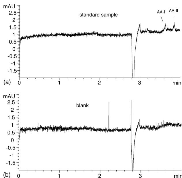
Fig. 4. Detection limits of AA-I and AA-II: (a) standard sample; (b) blank sample. Separation conditions: 120 mM borate buffer (pH 8.8) containing 10 mM  $\beta$ -CD, 50  $\mu\text{m}$  i.d.  $\times$  48.5 cm (40.0 cm effective) fused-silica capillary, applied voltage of 30 kV, capillary temperature of 10 °C, UV detection at 254 nm, injection at 50 mbar for 5 s. The concentration of each AA was 1.0  $\mu\text{g mL}^{-1}$ .
